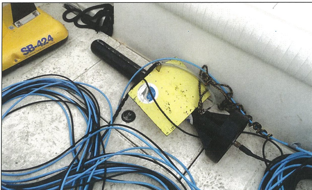
Marine Sonic Technology® HDS sidescan sonar with 600/1200 kHz towfish to be employed during the survey.
