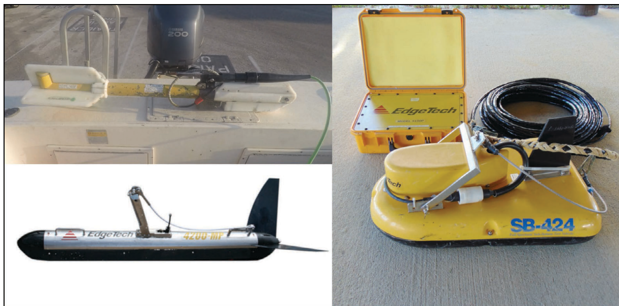
Figure 3-03. Survey instruments employed during the investigation included (clockwise from top left) the magnetometer, the subbottom profiler, and sidescan sonar.
