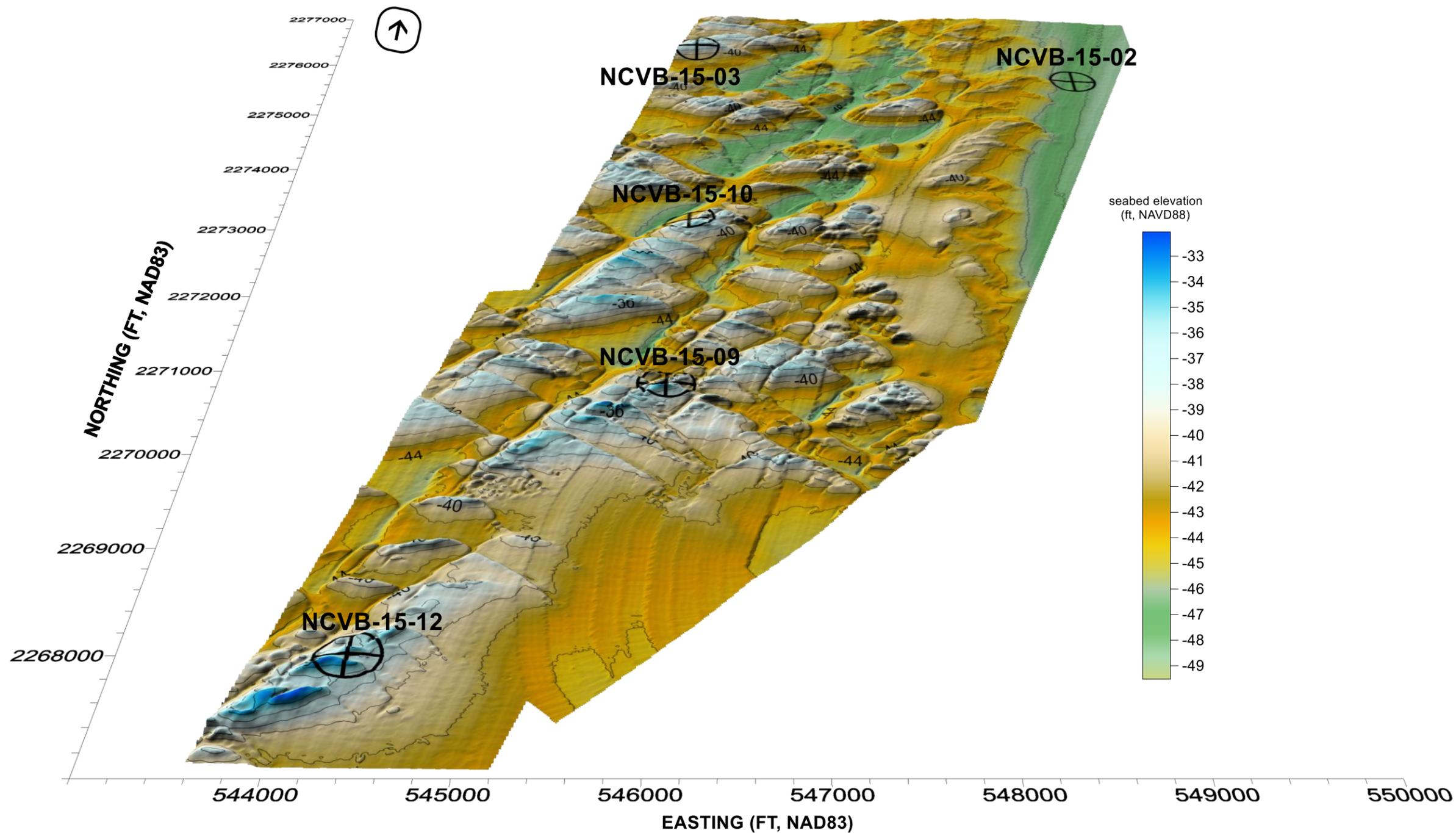
**Figure 4.2** 2015-2016 Multibeam survey map of the B5 shoal identified by Meisburger and Field (1975). The October 2015 Vibracores collected in the vicinity of the shoal are denoted in black.
