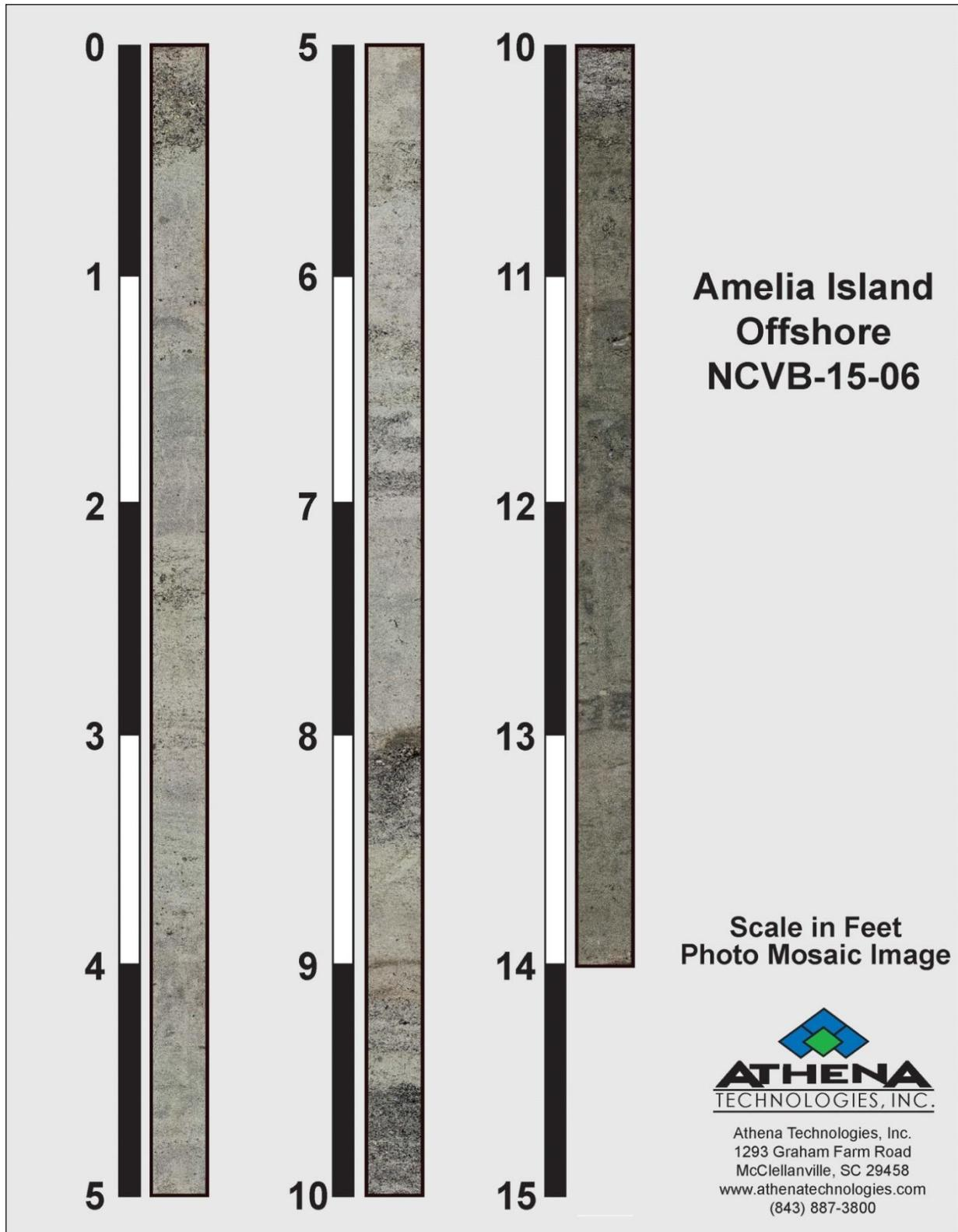
**Figure 5.2** Photo log of Vibracore #NCVB-15-06, collected in October 2015 on the B4 Shoal off Nassau County, FL (Meisburger and Field, 1975). The geotechnical log can be found in Appendix B.
