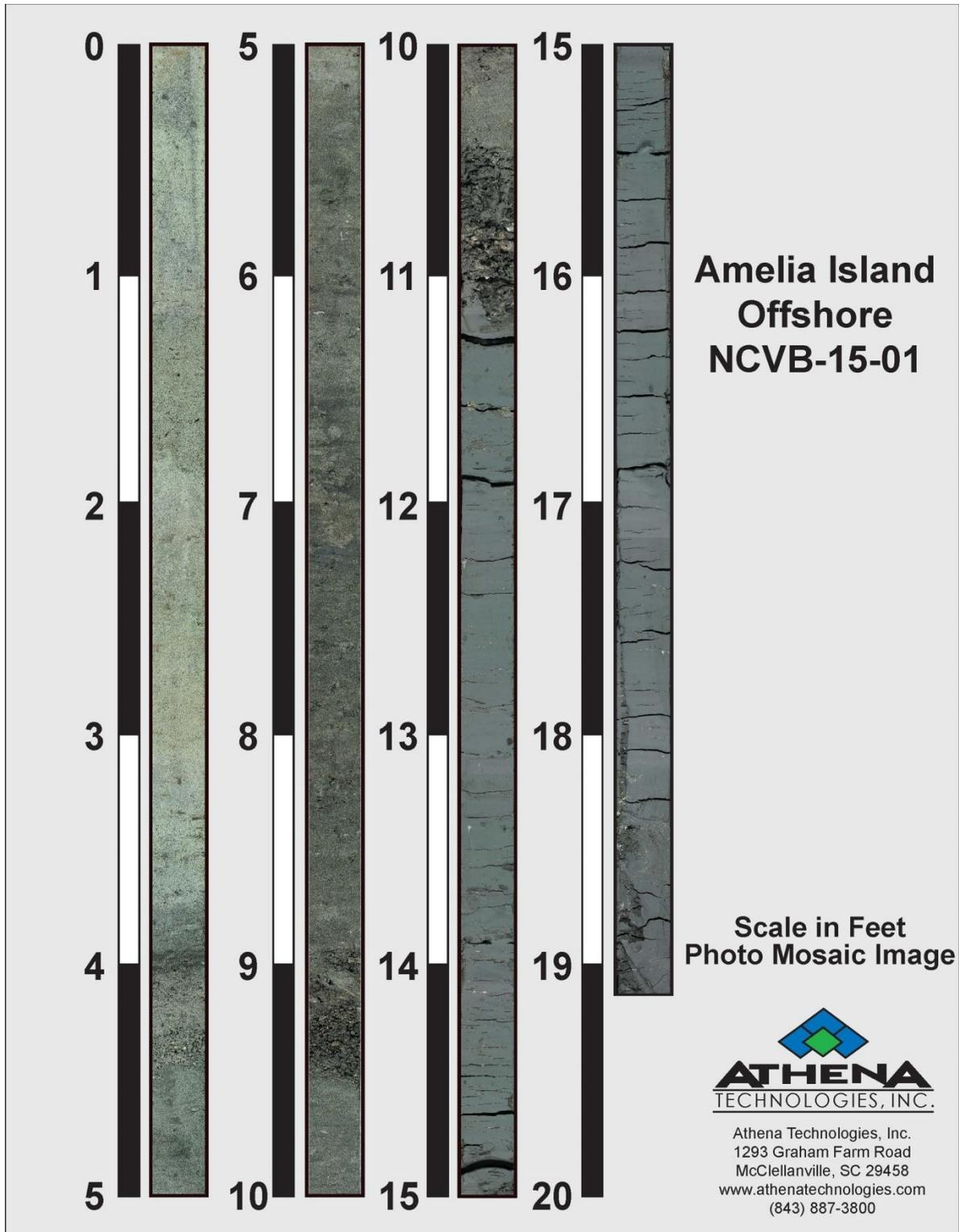
**Figure 3.2** Vibracore photographs of core NCVB-15-01, collected offshore Amelia Island in October 2015. Divisions are feet from the seabed to over 19 ft below the seabed. Note the transition from sandy or shelly sediments around 11 ft to stiff gray clay below.
