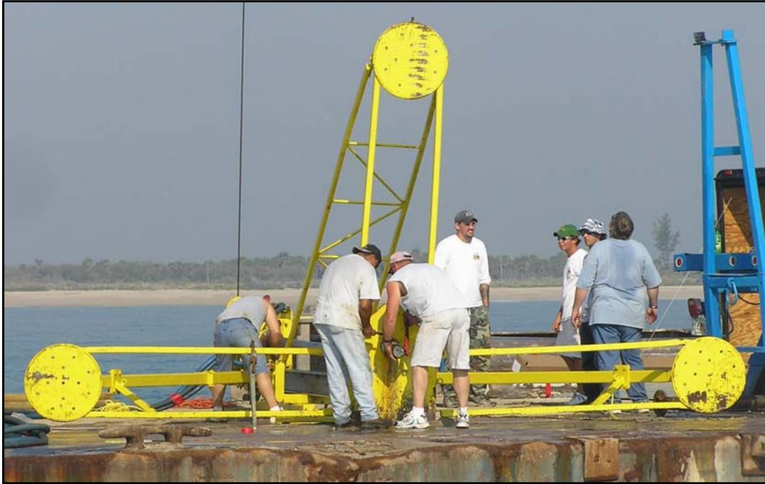
Figure 6. The 271B Alpine Pneumatic Vibracore unit.
