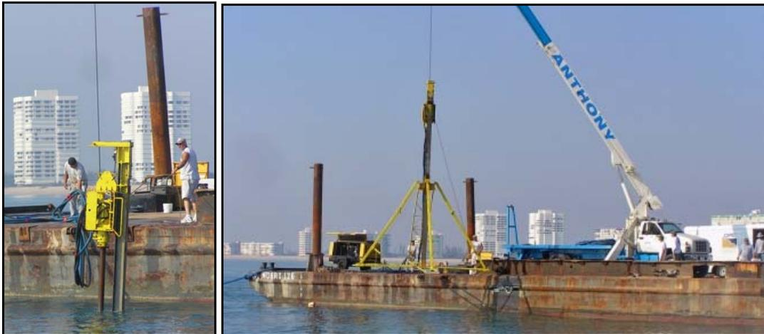
Figure 7. Core extraction from (top) and truck-crane deployment of (bottom left and bottom right) the 271B vibracore unit.
