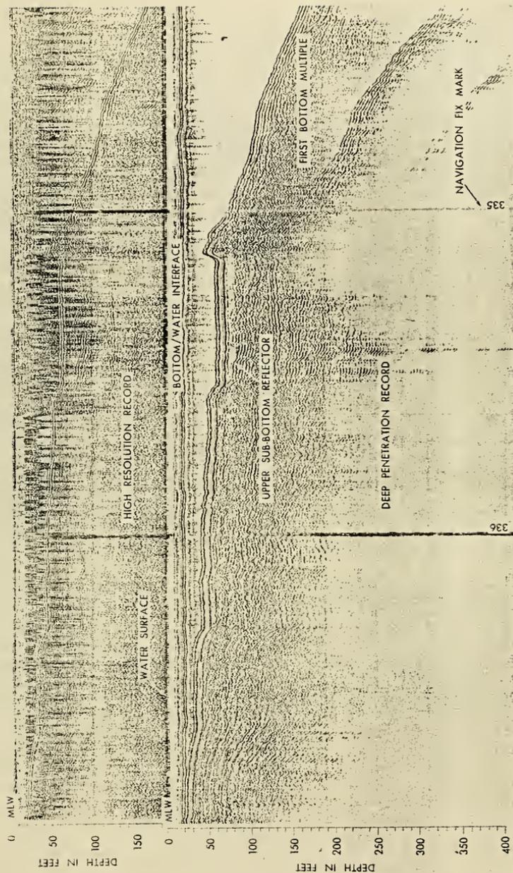
Figure 11. Typical dual channel marine seismic reflection record.
