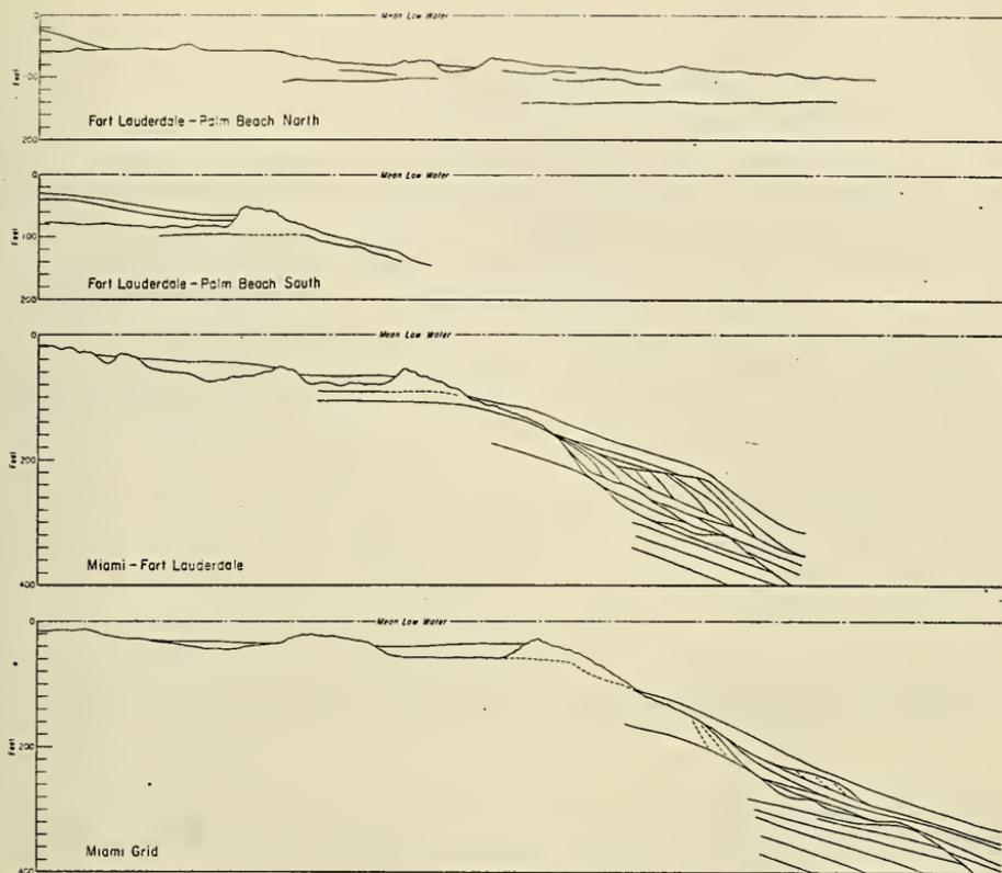
Figure A-4. Reduced seismic reflection profile data.
