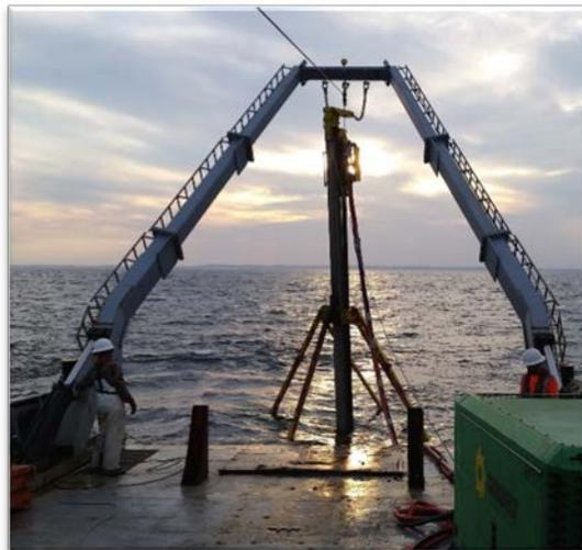
Figure 12: Alpine vibracore rig.
