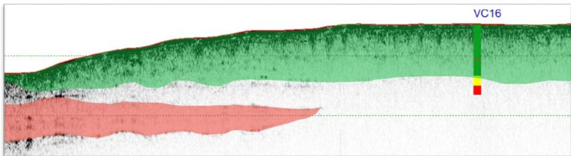
**Figure 14: Chirp sub-bottom Line 042 offshore St. Johns County. The brown line at the top of the sub-bottom record represents the seafloor. Layers color coded as green are likely beach compatible, yellow indicates potentially incompatible material, and red indicates likely incompatible material. The color-code criteria are further explained in the Reconnaissance Geologic Sample Data Interpretation section of this report.**
