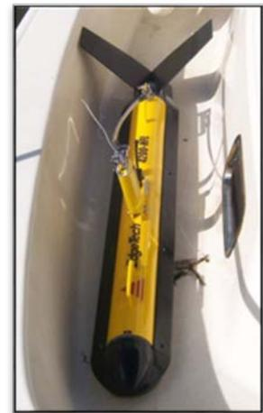
Figure 9: Image of the EdgeTech 4200 Sidescan Sonar towfish.
