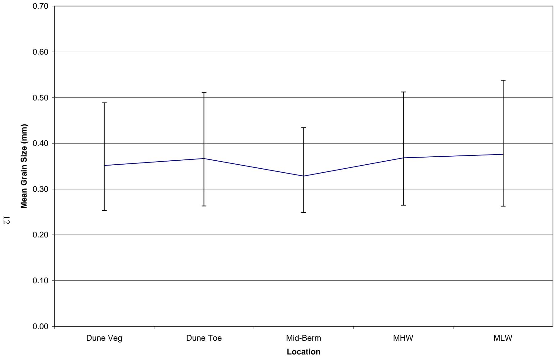
**Figure 3.2** Mean and Standard Deviation of Native Sand by Sample Location in Eglin AFB
