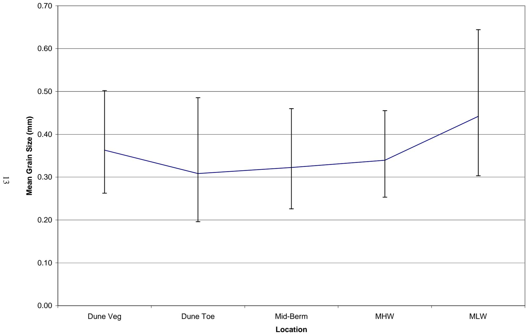
**Figure 3.3** Mean and Standard Deviation of Native Sand by Sample Location in Okaloosa Island
