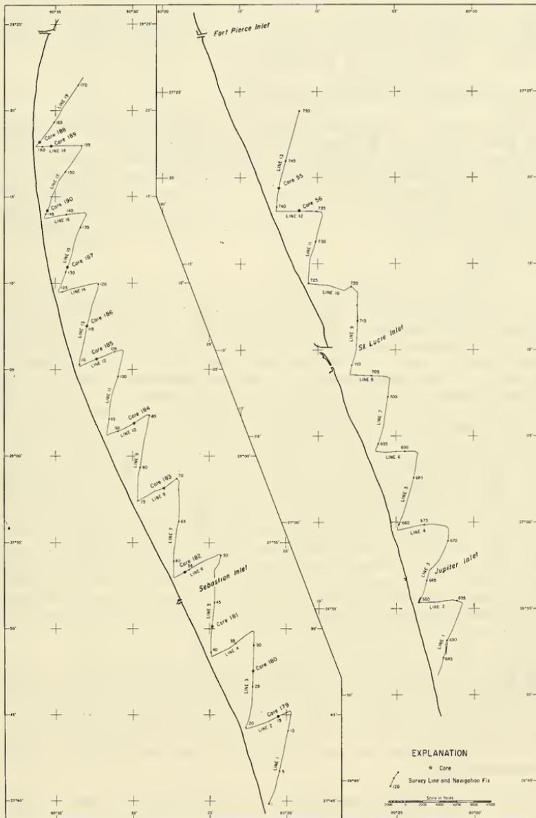
Figure 3. Navigation Plot Showing Survey Tracks and Core Locations in Reconnaissance Areas North (left) and South (right) of Fort Pierce Grid.
