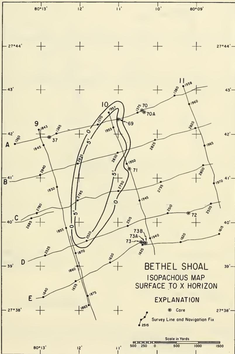
Figure 29. Isopachous Map of Sediment Thickness between the Water-Sediment Interface and the "X" Horizon Underlying Bethel Shoal.
