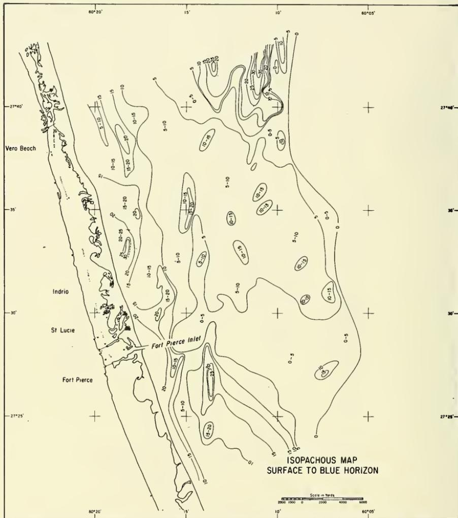
Figure 9. The Isopachous Map of the Interval from the Water-Sediment Interface to the Top of the Shallow Blue Acoustic Reflector. Shows a marked similarity to bottom morphology of the Fort Pierce Grid Area.
