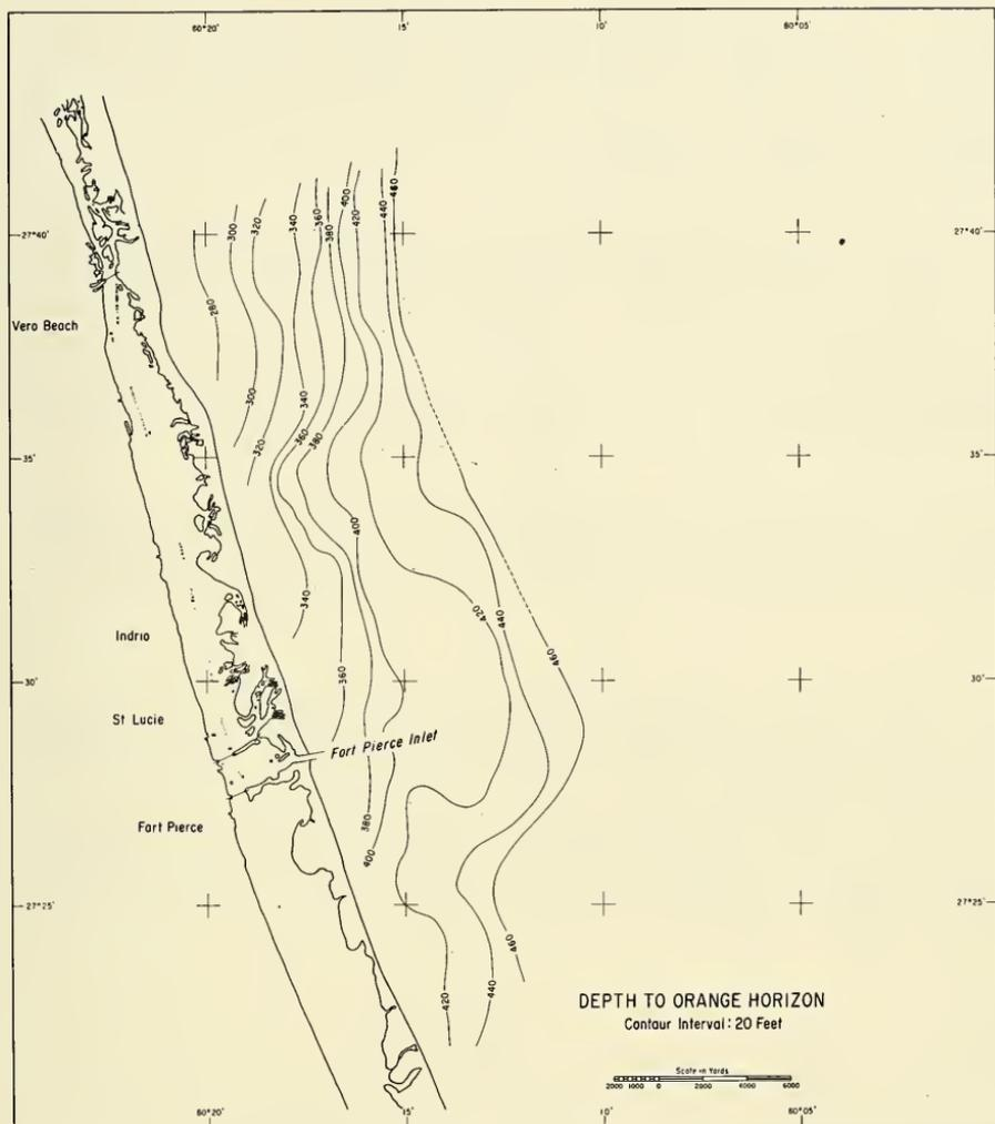
Figure 11. Contour Map of the Surface of the Orange Reflecting Horizon. Depths are in feet below MSL. Note change in dip and strike of this horizon compared to shallower yellow and blue reflectors (compare with Figures 10 and 8).
