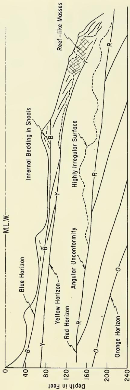
Figure 7. Schematic Profile Showing Characteristics of Prominent Shallow Acoustic Reflectors underlying the Bottom.
