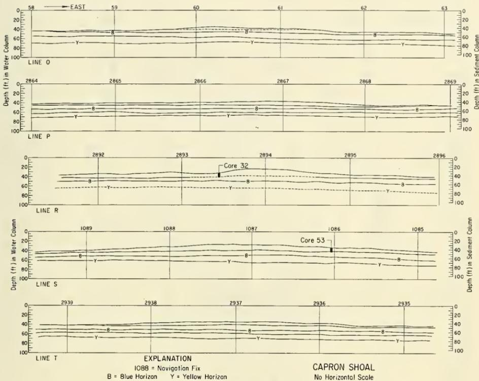
Figure 31. Line Profiles showing Horizons in the Capron Shoal Area.
