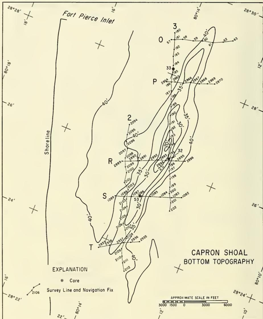
Figure 30. bottom Topography and Survey Control in the Capron Shoal Area. Capron Shoal contains sand considered suitable for beach nourishment.
