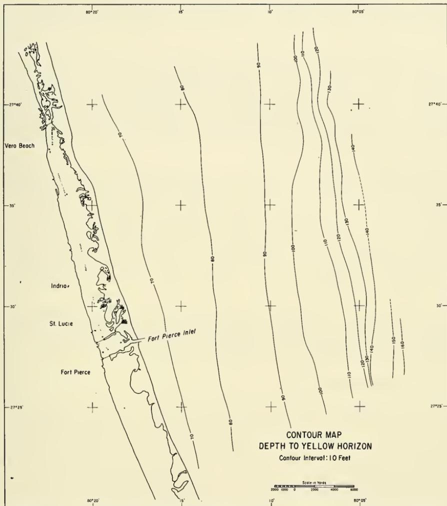
Figure 10. Contour Map of the Surface of the Yellow Reflecting Horizon, Depths are in feet below MSL. Note similarity of structure to the superposed "blue" horizon (compare with Figure 8).
