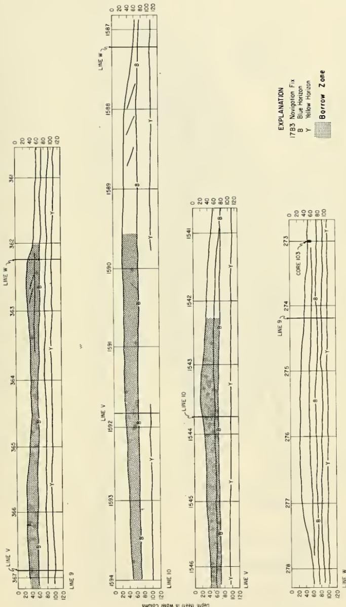
Figure 30. Interpreted Geophysical Profiles Across Representative Sections of Southeast Shoal
