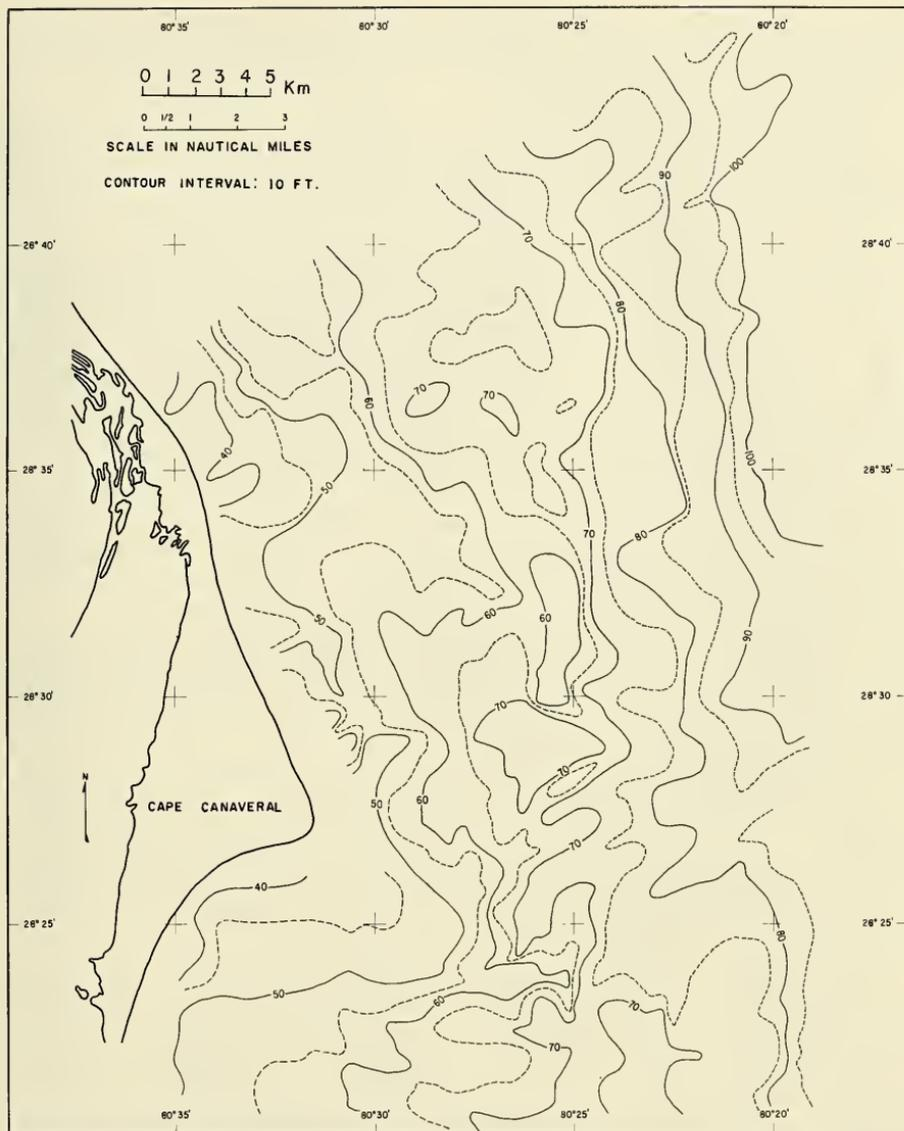
Figure 9. Structure Contour Map of the Blue Horizon in the Cape Canaveral Grid. Depths are in feet. Note similarity of surface configuration to that of the yellow horizon.
